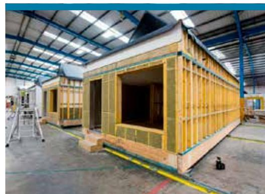
Manufacturing volumetric modules
