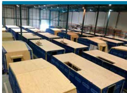
Volumetric modules manufactured offsite by AMK
