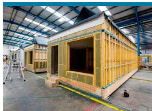
Manufacturing volumetric modules
